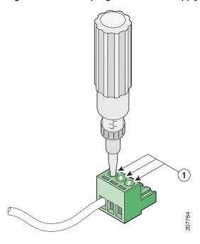
1 Torque is from 4.425 in.-lb (.5 N-m) to 5.310 in-lb (.6 N-m).
